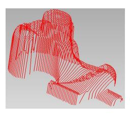
We can cross-section the scan and export the **curves** for modeling in native CAD packages (SolidWorks, Inventor, Pro-E, etc)
